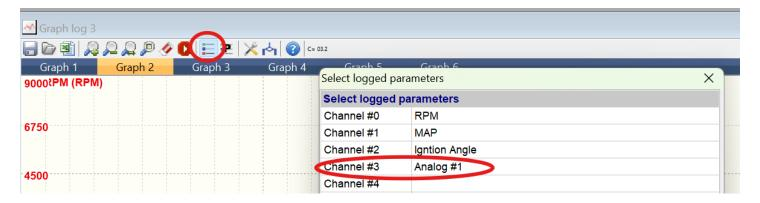
5 - You can now view your selected analog input in the datalogs. Remember the voltage will grow with RPM, but you're looking for sharp spikes in the amplitude indicating potential knock events.
