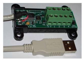
2 – Once you have your DLP-IO8 installed with the appropriate drivers, connect the **BLUE** wire from the Knock Detective to one of the 8 inputs. Splice in a ground wire from your Knock Detective to the GND pin on the DLP-IO8.
